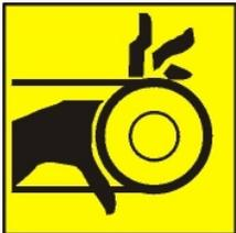
This warning symbol alerts you to the presence of possible dangerous drive mechanisms within the machine. Guards should always be in place when the machine is in operation. Be careful when servicing any drive mechanism.
