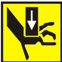
This warning symbol indicates the presence of possible dangerous pinch-points. Moving mechanical parts can crush an/or sever body parts.
